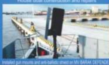
Installed gun mounts and anti-aircraft shield on MV SARAK DEFENDER
